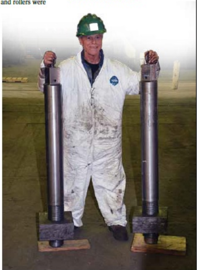
JIM BAYS PROUDLY SHOWING OFF THE NEWLY COMPLETED JACK SCREWS. THE ENTIRE WEIGHT OF THE TABLE SITS ON THESE SCREWS.
